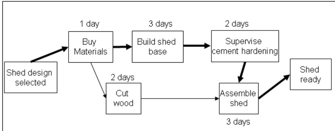
The above network diagram shows the relationships (arrows) between the main activities (rectangles) that are required to build a shed. You can flesh out the following information from the above diagram:
